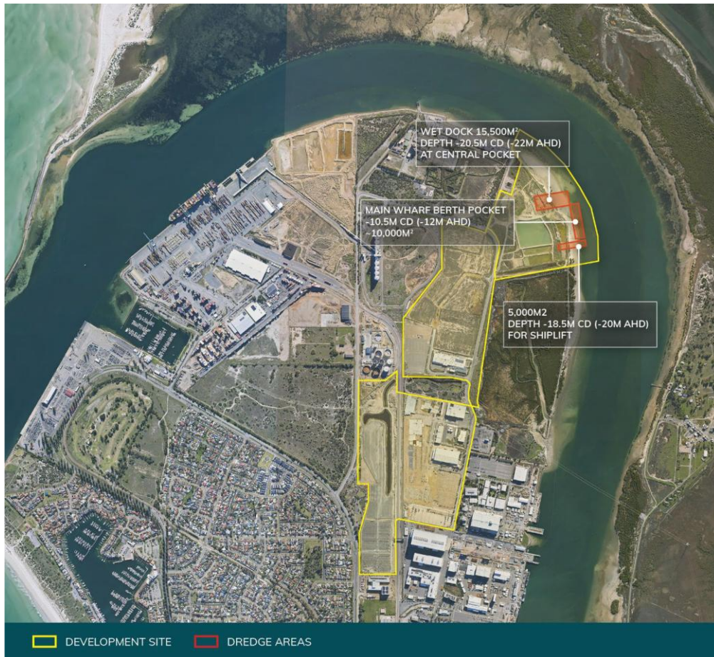
Figure 5.1 - Preliminary dredging areas for the construction of the development, Appendix 1.17
